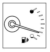
The fuel gage shows approximately how much fuel is in the fuel tank. It works only when the engine is on.
